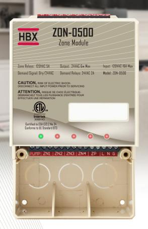
The ZON-0500 is an intelligent, microprocessor based zone control. Capable of controlling up to 4 zones per control, the ZON-0500 can be used as a standalone unit, in conjunction with the 0550 series or as an expansion module for the 1000 series controls, and can handle multiple priority selections.
