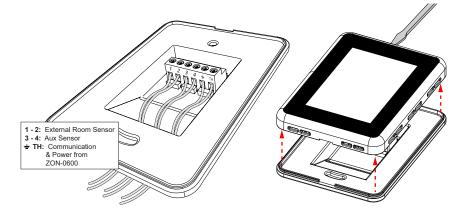
In order to assure proper room temperature, it is important to identify the ideal location of the thermostat. It should be approximately 5 feet from the floor and at least 1 foot from door openings on an interior wall. Avoid exposing the thermostat to direct sunlight, to air flows (doors, windows, etc.) as well as to heat sources. Ensure the cavity that the thermostat will be installed in is well insulated.
