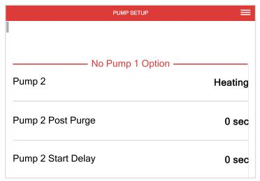
When four (4) heat pumps and a backup boiler is selected there will be no pump 1 option as the pump 1 relay will be controlling the backup boiler.
