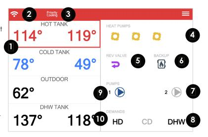
Accessing the menu of the ECO-0600 is done by pressing the menu button (3 lines) in the top right corner.
