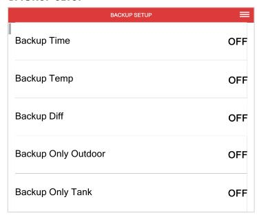
**Backup Time** - This setting will be set for the minimum lag time between heat pump stages and the backup boiler. This is a time delay between the heat pump stages and the backup boiler. The backup time can bring on the backup even if differential and temperature are not in their range so long as the backup time has elapsed.
