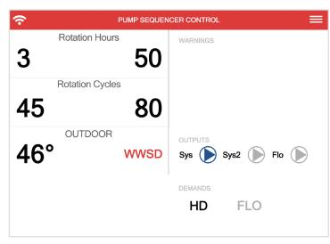
If the box is outlined in orange that indicates there is a no flow warning for pumps 1 or 2. After 10 attempts to start the pump the box will be outlined in red and will trigger the flow alarm.
