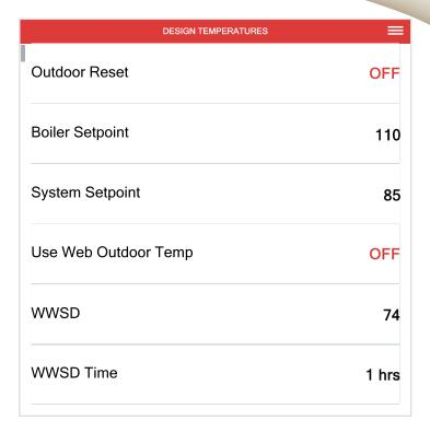
If the control disconnects from the Wi-Fi after 2 hours or longer it will go to the coldest day of the year set in your outdoor reset design or maximum boiler temperature.
