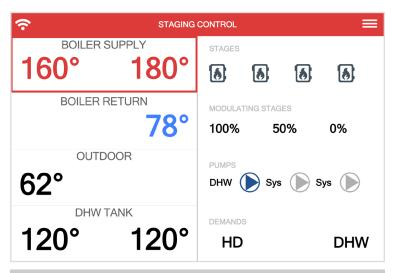
In the event you select the wrong control mode, please cycle power to the controller and it will display the control mode option screen.
