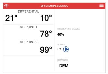
Accessing the menu of the CPU-0600 is done by pressing the menu button (3 lines) in the top right corner.
